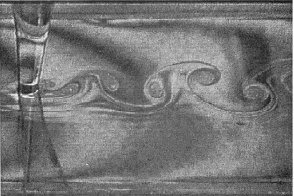
FIGURE 22. Flow visualization by soap film. (a) A water jet injected through the soap film shows no structure in the wake; (b) the jet nozzle inserted through the soap film sheds vortices.
