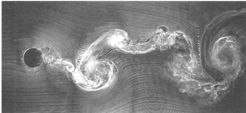
FIGURE 11. Cross-sectional views of jet wakes. Re_{cj} = 7600 . (a) V_R = 4 , Z_{sw}/D_j = 1 ; (b) V_R = 6 , Z_{sw}/D_j = 0.25 ; (c) V_R = 6 , Z_{sw}/D_j = 0.5 .
