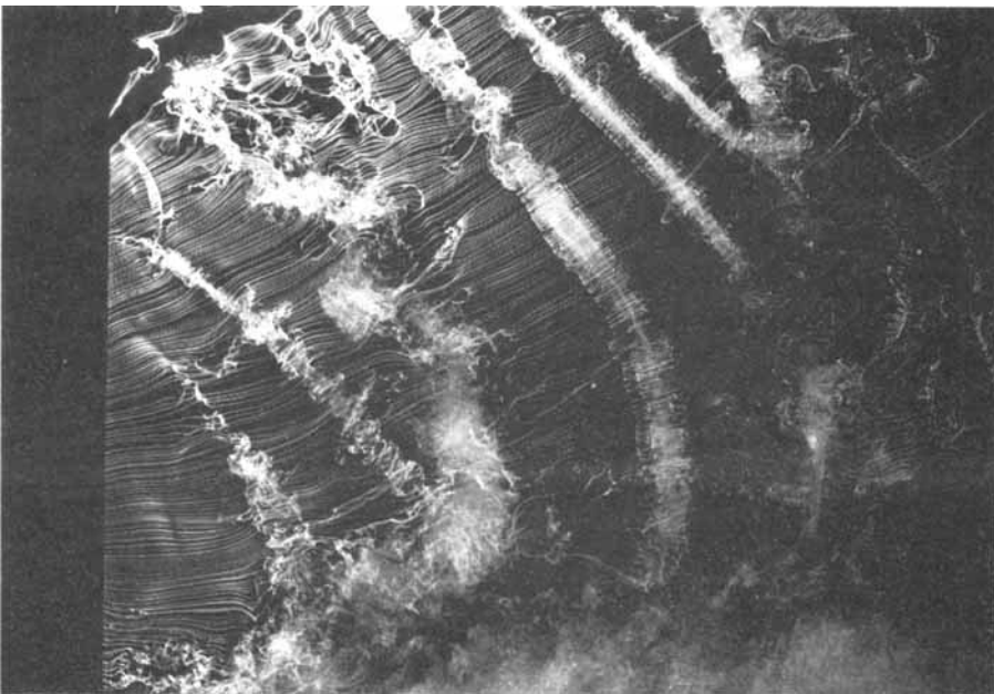
FIGURE 15. Side views of wake vortices with smoke injected directly into the wake. (a) V_R = 8 , Re_{cf} = 3800 , X_{sw}/D_j = 2 , Y_{sw}/D_j = -0.5 ; (b) V_R = 10 , Re_{cf} = 11400 , X_{sw}/D_j = 6 , Y_{sw}/D_j = 0 .
